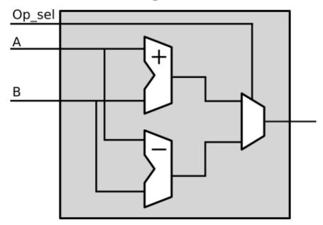
If the RTL is unfamiliar, the two leftmost components are ALUs which do arithmetic (addition and subtraction in this case) The rightmost component is a multiplexer which selects an input signal based on a selector signal, kind of like a railroad switch.
